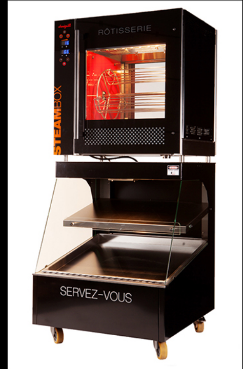
NEOBOX Electric W: 33 3/4" D: 37 3/4" H: 78 3/4" 4 Baskets - 16 chickens/hour 220 V Triphase - 11.6 Kw - 30.6 Amps
