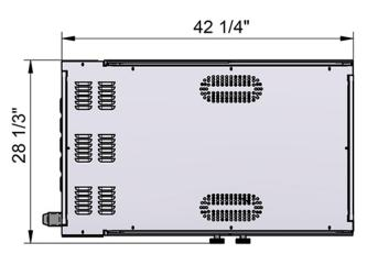
Power = 10kW Plug = 52A 220V triphase +T+N
